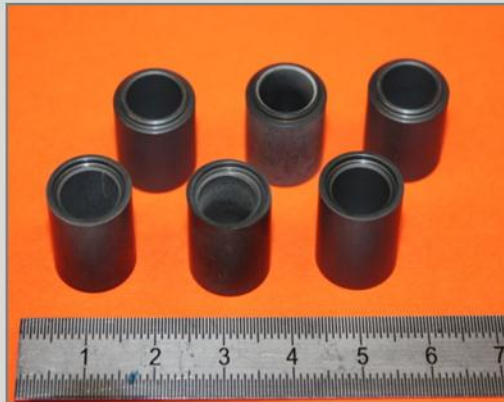
SSiC- capsules StarCeram S (H.C.Starck) Ø: 12 mm, h: 16 mm
